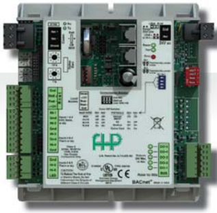
DDC Control Board
