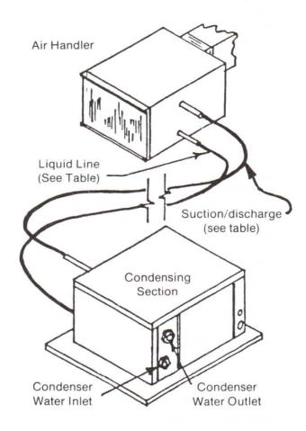
After the interconnecting refrigerant lines have been installed, the entire system should be pressurized with R22 and leak checked. Then, using a good vacuum pump, evacuate the system for a minimum of six (6) hours, then charge in accordance with Tables 1 and 2 in the following instructions.
