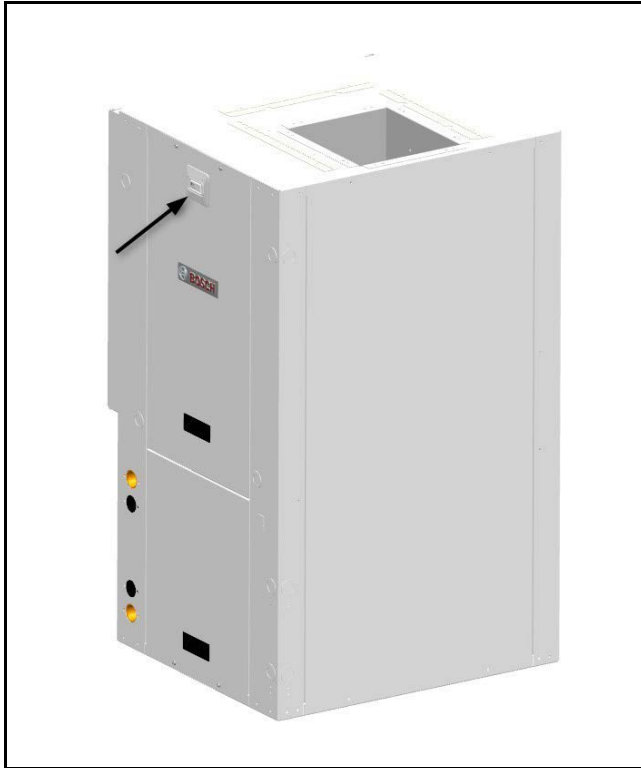
Fig. 69 Vertical (VT) Unit WIM Mounting Location
