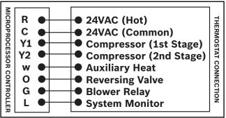
Figure # 15 Thermostat Wiring
